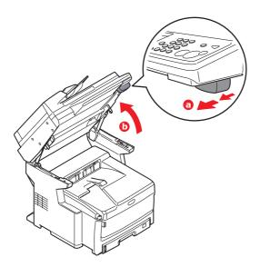
**2.** Press the cover release (a) and open the top cover (b) fully.
